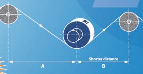
To obtain the maximum spreading effect the distance travelled between the spreader and the following roll (B) must be as short as possible.
