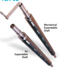
Core holding is initiated mechanically and not pneumatically in this lug type shaft. Excellent performance is delivered even for heavy load and higher speed. Positive gripping and core centering are achieved with the help of cam/lug design. Easy handling of cores with uneven inside diameter. Key and alien cap bolt prevent any shearing of journals pipe assembly.
