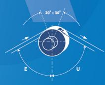
Normally, the entering angle (E) and the leaving angle (U) are set equal. by adjusting spreader roll position.
